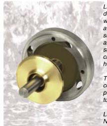
L50 Series inducer style pumps are designed specifically for applications where the net positive suction head available at the pump inlet is limited, such as in boiler feed water deaerator and refrigerant services. A centrifugal style impeller with good low NPSH characteristics is utilized to lower the inlet head requirements.
