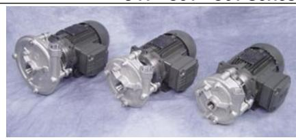
units also make use of our custom manufactured D3 dual face motors found on our T31, E41, and E51 turbine pumps, and feature a stainless steel shaft and a heavy duty front motor bearing. D3 Motors also feature UL and CE approvals. The C Series standard construction is investment cast 316 SS casings and impellers with Viton elastomers. Options - See below.
