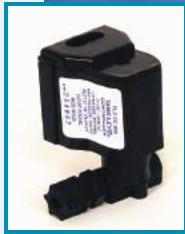
Our TLC Series utilizes a switch/valve combination which automatically shuts off feed water at a predetermined "full level" and then reopens the integral feed water valve at a second "refill level". The TLC Series provides a switched output to control a pump or other accessory.
