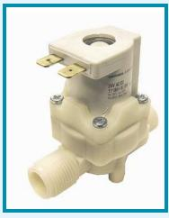
Aquatec's ESO Series (ESO 460, ESO DC100, ESO High Flow) are normally closed, precision solenoid valves that positively shut off feed water. They are activated by a pressure switch to either open or close at predetermined holding tank pressure settings. The ESO Series can either be used independently or mounted inline on the inlet side of a pump. Our ESO Series also includes a modular connector for plug-and-play integration with Aquatec's other system components.
