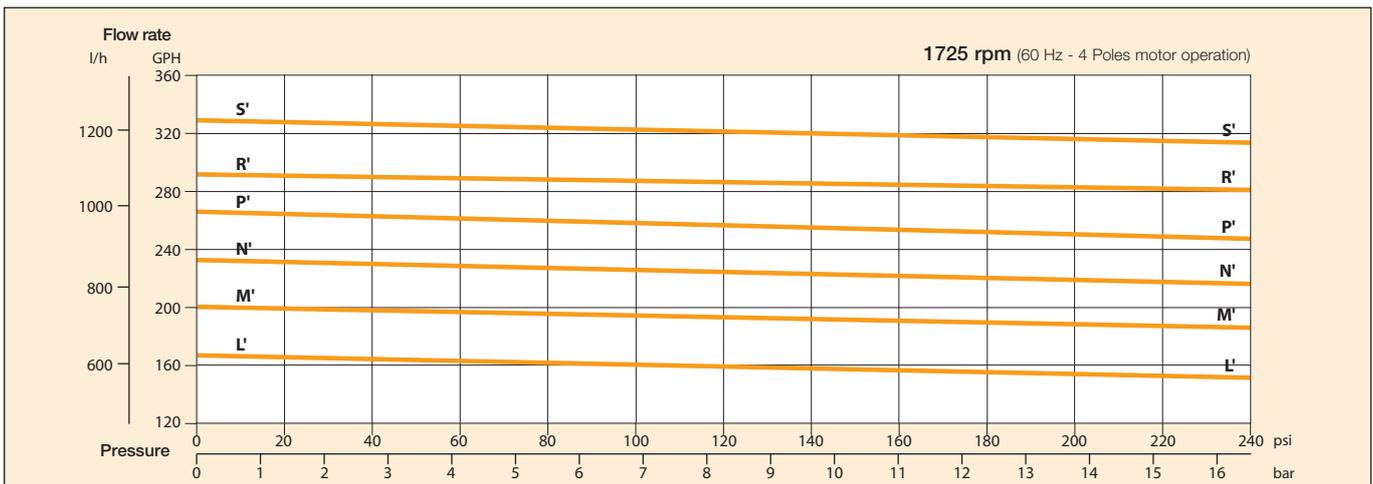
Note: Characteristics at constant motor speed, with water at 20 °C (68 F) and bypass blocked - Figures of flow are averages.
