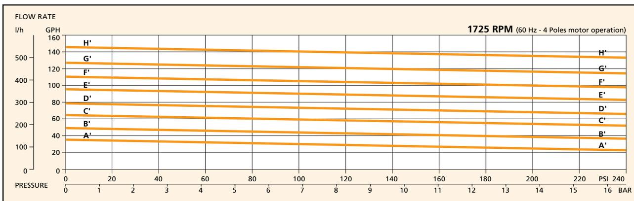
Pump weight: 1,1 kg / 2.5 Lbs (clamp mount) 1,2 kg / 2.7 Lbs (flange mount) - Characteristics at constant motor speed, water at 20 °C / 68 °F and by-pass blocked
